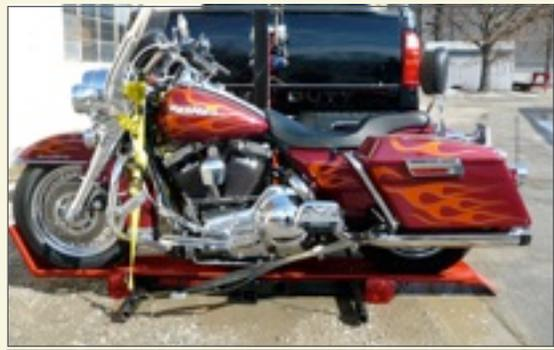
We recommend that this hauler be used by vehicles with a class IV or V hitch. The heavier the hitch the better. The receiver size needs to be 2" square or else you need a receiver reducer. Please consult with your vehicle or hitch manufacturer for complete requirements and specifications for your specific hitch.
